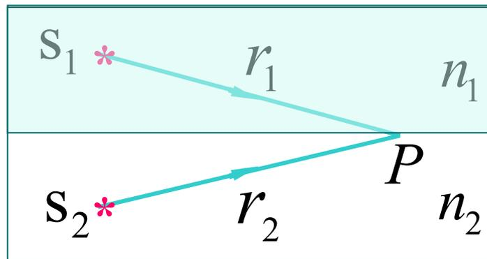
✓ 干涉加强  $\left\{ \begin{array}{l} \Delta = \pm k\lambda, \quad k = 0, 1, 2, \\ \Delta\varphi = \pm 2k\pi, \quad k = 0, 1, 2, \end{array} \right.$
