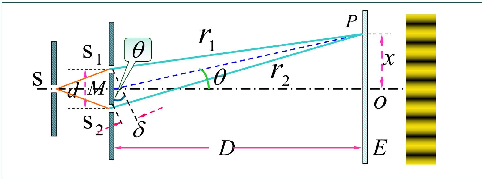
$$d \frac{x}{D} = \delta = r_2 - r_1 = \begin{cases} \pm k \lambda & \text{干涉加强} \\ \pm(2k-1) \frac{\lambda}{2} & \text{干涉减弱} \end{cases} \quad k = 0, 1, 2,$$
