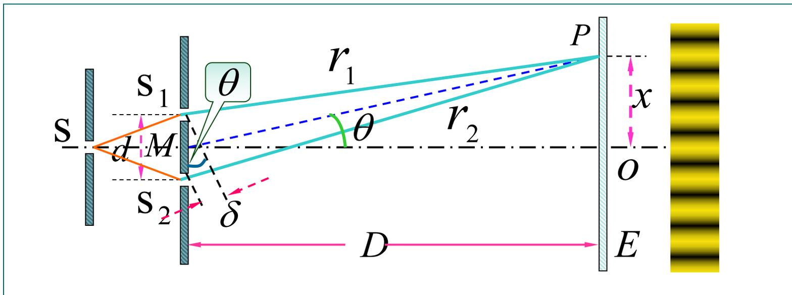
$$\delta = r_2 - r_1 = \begin{cases} \pm k\lambda & \text{干涉加强} \\ \pm(2k-1)\frac{\lambda}{2} & \text{干涉减弱} \end{cases} \quad k = 0, 1, 2,$$
